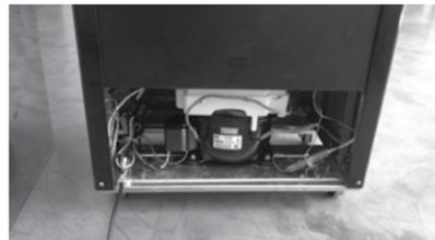
3. Replace or service the parts in the compressor compartment.
