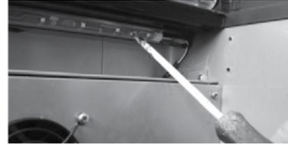
**3** Using a Phillip's screwdriver, remove the (2) screws securing the LED light strip.
