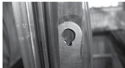
4. Align the rod so that the notch is aligned with the notch on the pin and it can now be pulled free.
