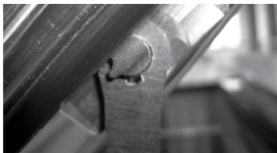
3. Remove the tension rod from its pin (the rod will remain connected on the lid).
