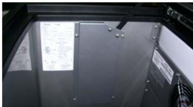
1. Using a Phillip's screwdriver remove the (6) screws from the left tension rod cover.
