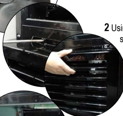
2 Using a small Phillips head screwdriver, remove the three screws as shown.
