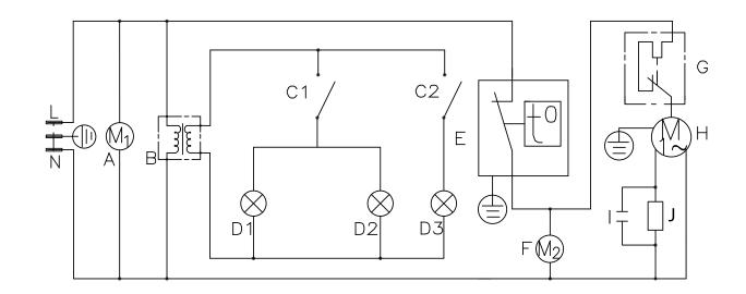
A. Evaporator Fan B. Power Supply for LED Lights C1. On/Off Switch for Interior Light C2. On/Off Switch for Canopy Light D1. Interior Top LED Light D2. Door Side LED Light D3. Canopy LED Light
