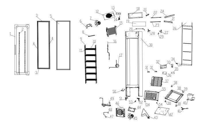
1. Glass Door 2. LED Light inthe Glass Door 3. Upper and Lower Sides LED Light Cover (2) 4. Left and Right Sides LED Light Cover (2) 5. Door Gasket 6. Evaporator Fan Baseboard 7. Evaporator Fan 8. LED Light 9. Pilaster (4) 10. Shelf (6) 11. Shelf Clip (28) 12. Control Panel 13. Thermostat Panel 14. Thermostat 15. Evaporator 16. Return Pipe 17. Muffler Connecting Pipe 18. Canopy 19. Canopy Sign
